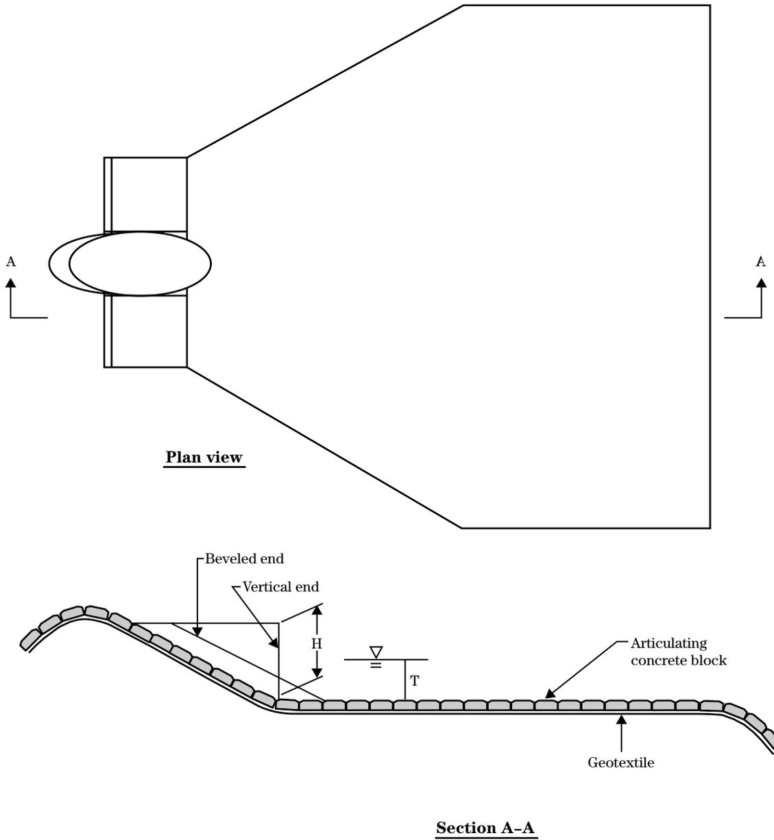
**Figure TS14L-6** Scour protection around bridge pier plan
