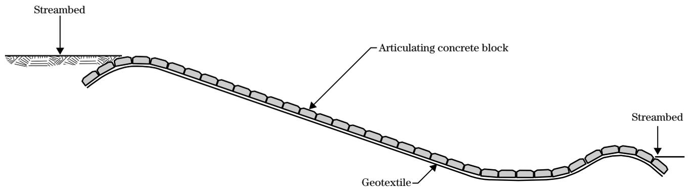
**Figure TS14L-5** Armoring of pipe/culvert outlets profile
