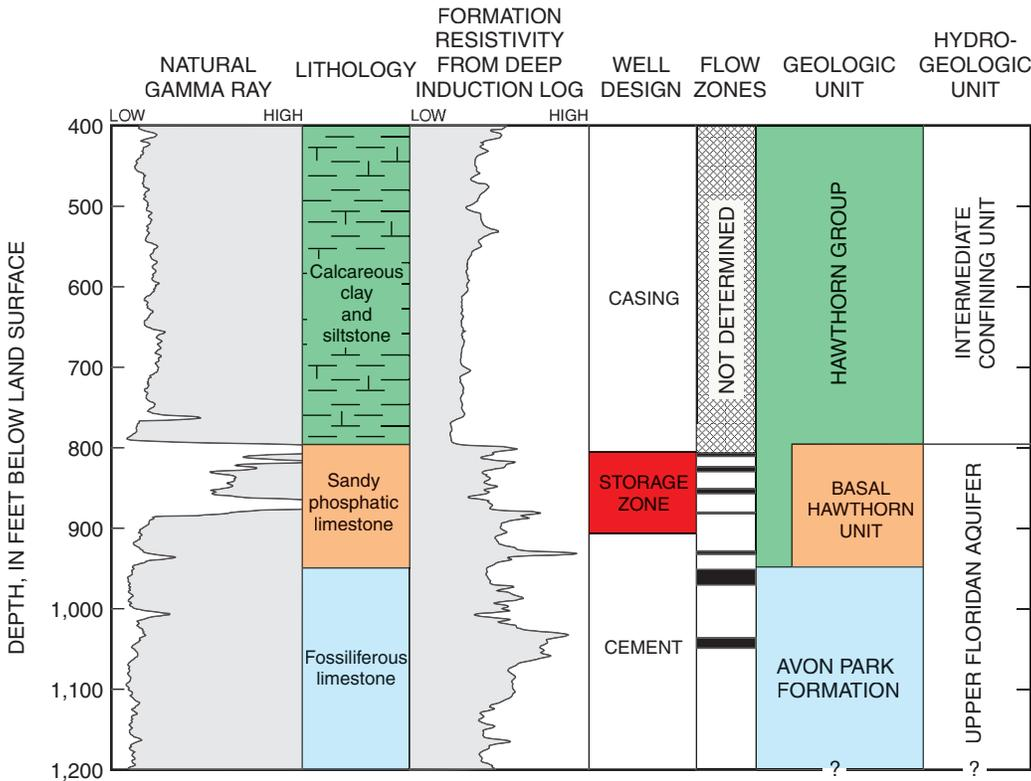
**Figure 3.** Location of storage zone in relation to geophysical logs, lithology, flow zones, and geologic and hydrogeologic units for the aquifer storage and recovery well at the Boynton Beach East Water Treatment Plant site in Palm Beach County. Flow zones determined by flowmeter, fluid resistivity, and caliper logs. The basal Hawthorn unit could include the Suwannee Limestone in its lower part. Question mark signifies that the base of a unit was not reached.
