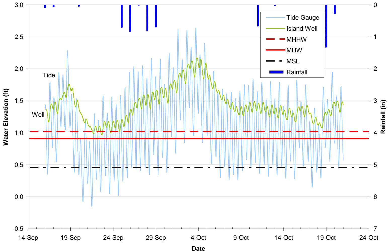
Figure 3: Recorded seasonal high water levels at Stuart, FL (September 2003). MSL, MHW, and MHHW are referenced to NGVD-29 and are based upon Tidal Epoch 1983-2001.
