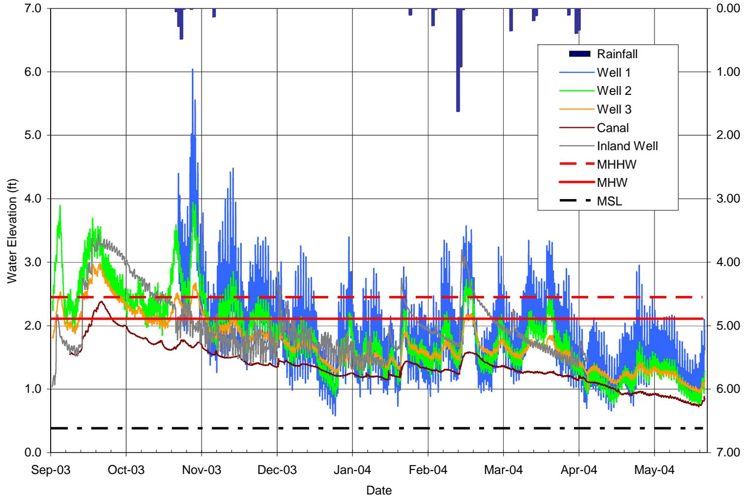
Figure 8: Recorded water levels at Cape Canaveral AFS (September 2003 to May 2004). MSL, MHW, and MHHW are referenced to NGVD-29 and are based upon Tidal Epoch 1983-2001.
