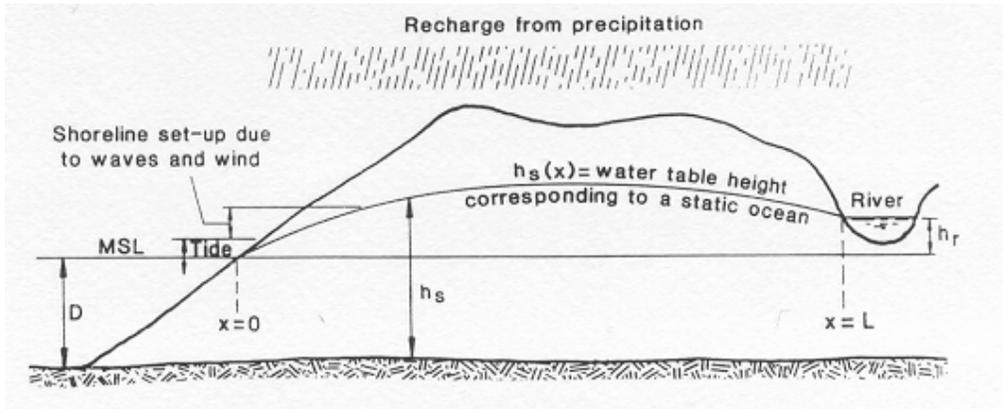
Figure 13. Estimated water table height corresponding to a static ocean (no waves) (From Nielsen, 1999).
