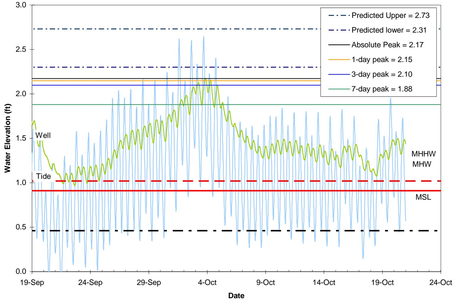
Figure 14: Comparison of predicted and observed peak water levels for Stuart, FL (September 2003).
