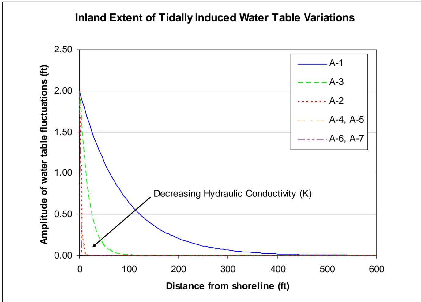
Figure 15. General estimates for the inland extent of tidally induced water table variations as a function of AASHTO soil classification. Assuming tidal amplitude of 2 ft and an aquifer depth of 25 ft.
