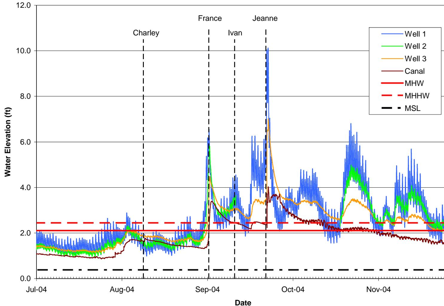
Figure 11: Recorded extreme high water levels at Cape Canaveral AFS (May 2004 to April 2005). MSL, MHW, and MHHW are referenced to NGVD-29 and are based upon Tidal Epoch 1983-2001.
