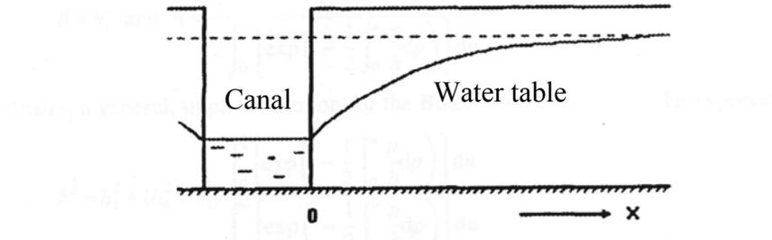
Figure 18: Water table elevation with respect to canal water levels.
