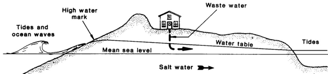
Figure 12: Combined effect of tides and ocean waves on water table elevations. The water table under coastal barriers will be highest near the ocean because of the action of waves and tides. Consequently there is a net flow of groundwater towards the continent and the fresh water lens tends to be very thin (From Nielsen, 1999)
