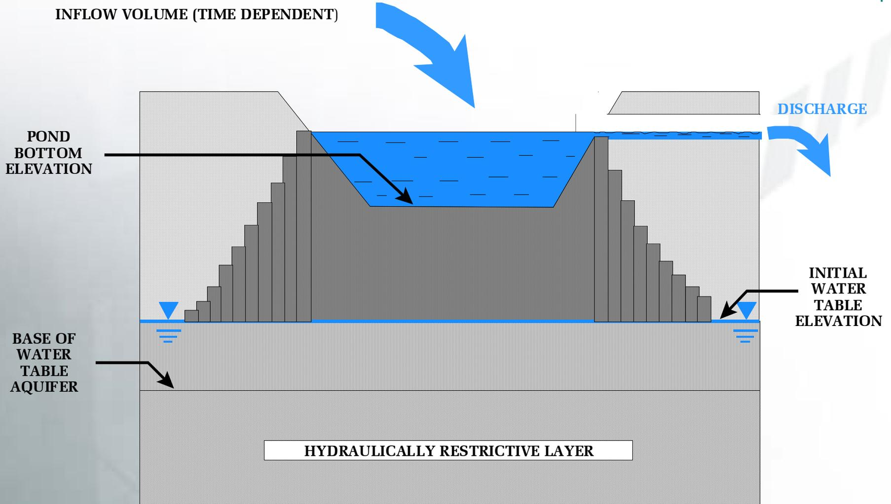
**note:** initial flat water table assumption is not unrealistic when the natural gradient is considered together with the duration of loading and the corresponding radius of influence.
