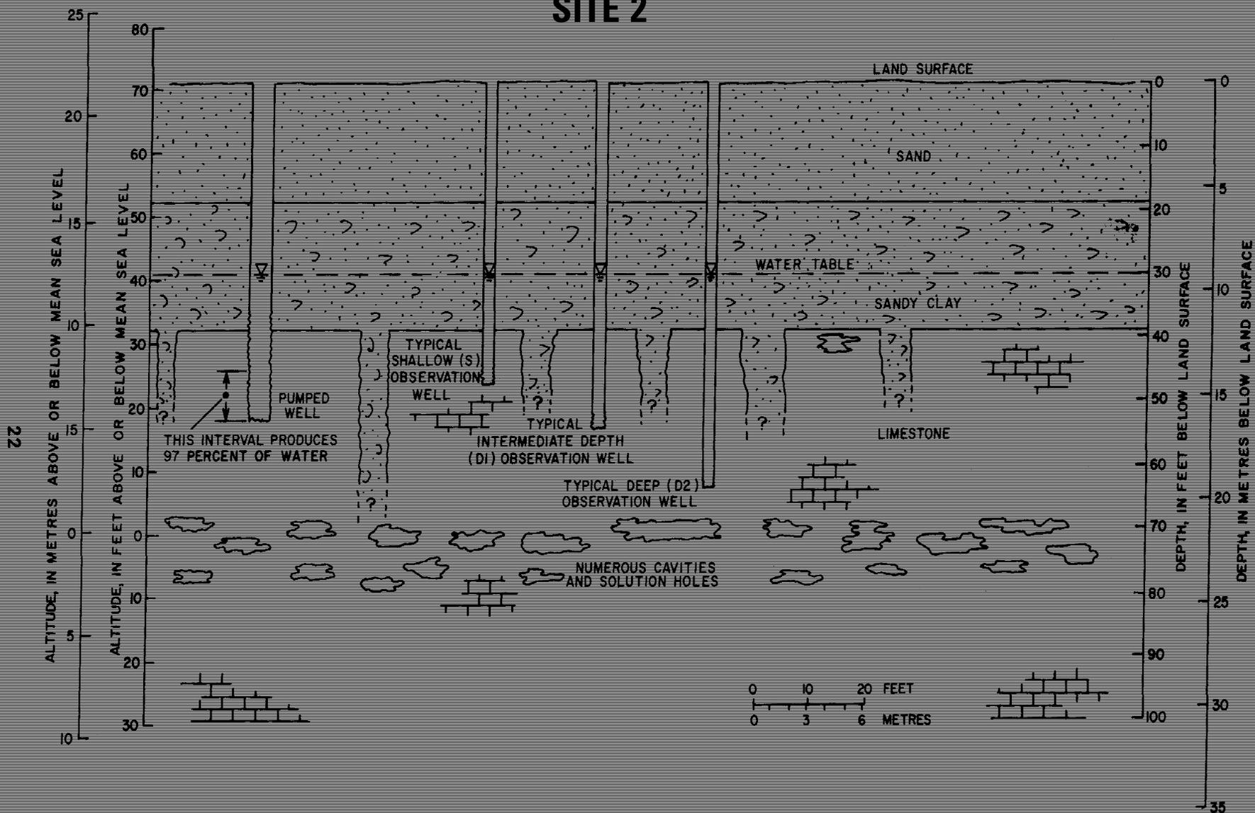
FIGURE 10:--SECTION SHOWING GENERALIZED GEOLOGY AND WELL CONSTRUCTION OF PUMPED WELL AND TYPICAL OBSERVATION WELLS AT AQUIFER TEST SITE 2.
