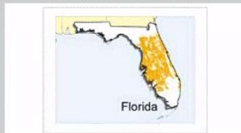
Myakka - This soil is poorly suited to urban development. Wetness is a management concern. Septic tank absorption fields can be maintained above the seasonal high water table by mounding and backfilling with suitable fill material.
