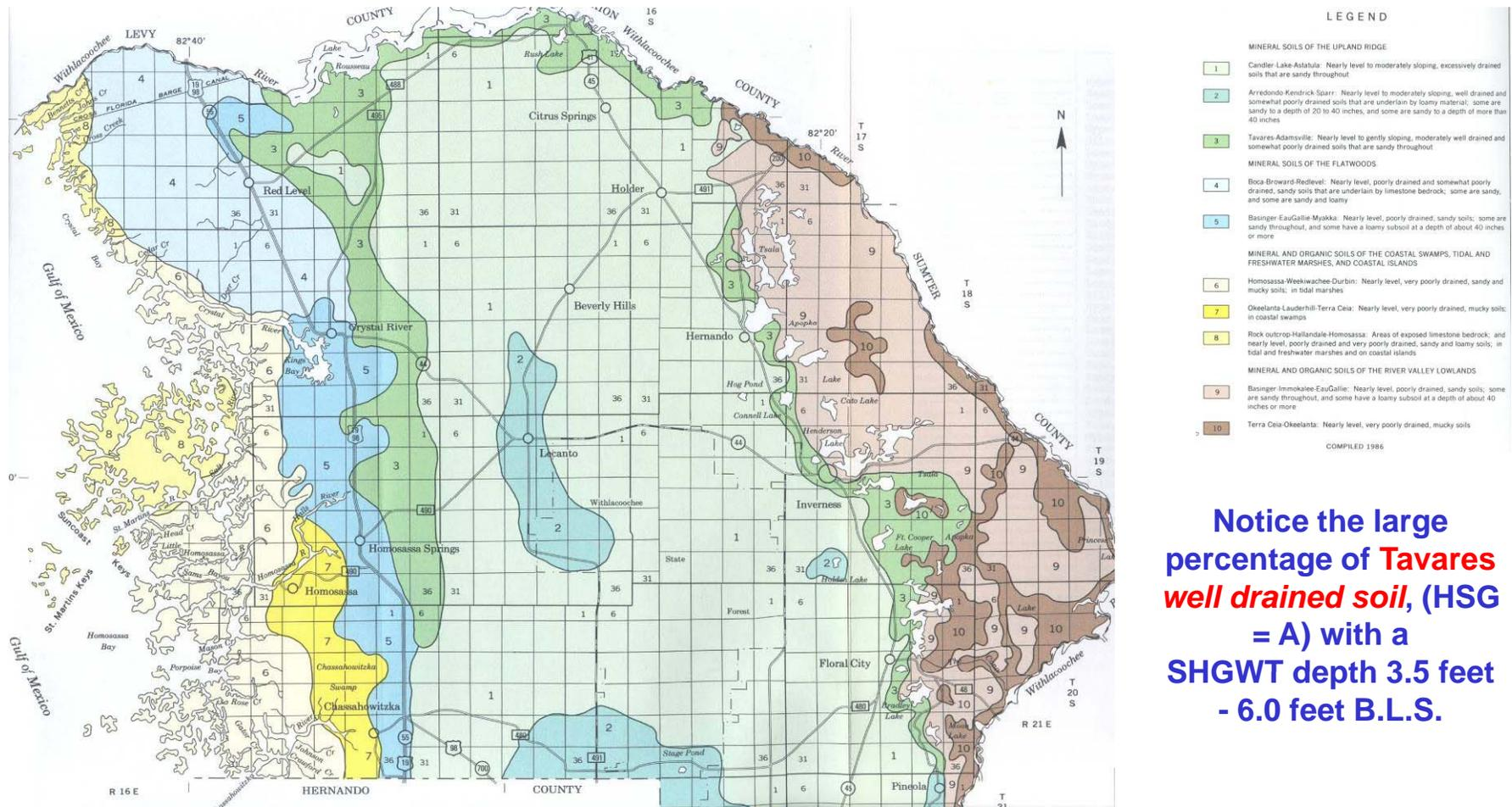
Notice the large percentage of **Tavares well drained soil, (HSG = A)** with a **SHGWT depth 3.5 feet - 6.0 feet B.L.S.**
