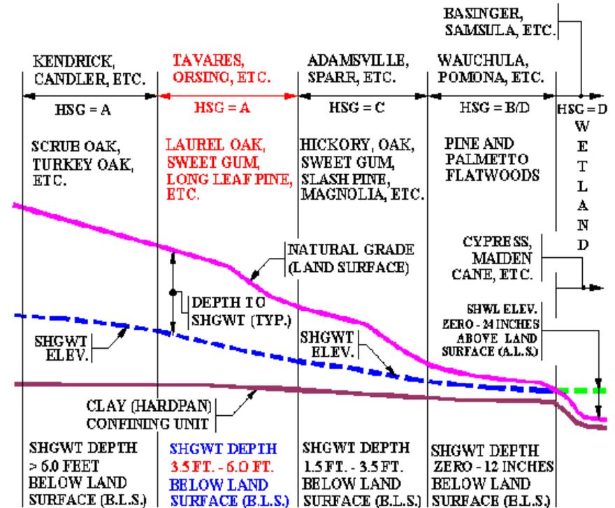
Notice the **change in upland vegetation**, and a **thicker ground cover**. Tavares is a well drained soil, with a higher SHGWT elevation.
