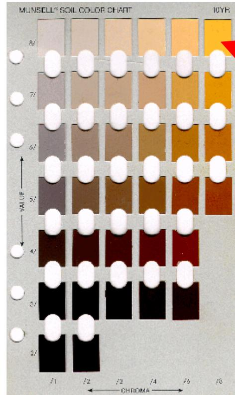
Excessively drained, HSG = A soils typically fall in this area of the 10YR page.
