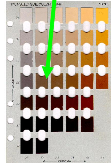
10YR page. Upper right corner indicates excessively drained soils (HSG = A), lower left corner indicates wetlands (HSG = D).
