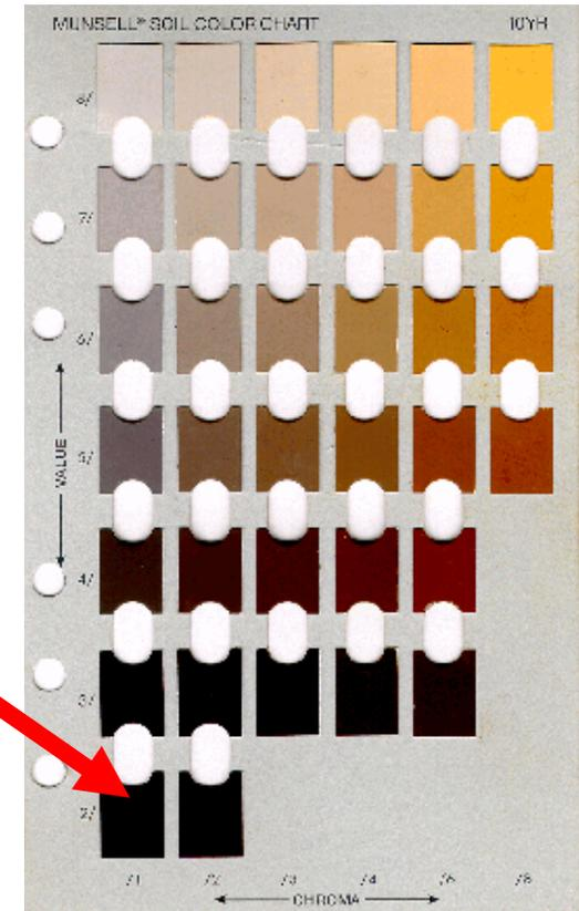
10YR page. Upper right corner indicates excessively drained soils (HSG = A), lower left corner indicates wetlands (HSG = D).
