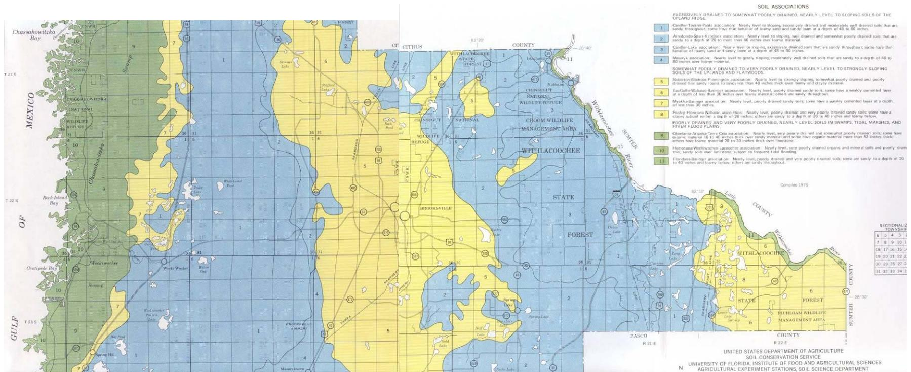
Note that a large portion of Hernando County contains **Nobelton / moderately to somewhat poorly drained soil** (HSG = C) with a **SHGWT > 1.5' – 3.5' B.L.S.**
