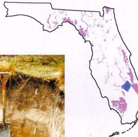
**Alfisols are typically classified as moderately drained, HSG = C, with a SHGWT between 1.5' to 3.5' B.L.S.**
