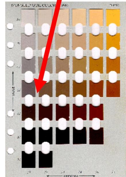
10YR page. Upper right corner indicates excessively drained soils (HSG = A), lower left corner indicates wetlands (HSG = D).
