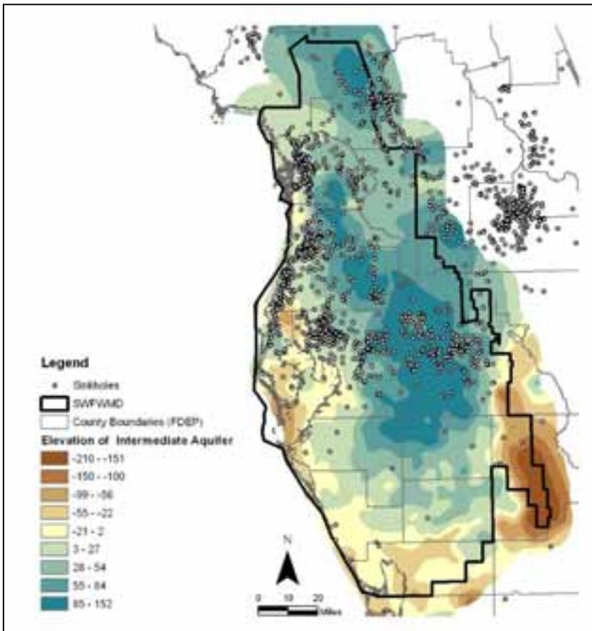
**Figure 2 – Top of Intermediate Aquifer**
