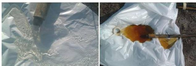
**Figure 3.** Flush water from treatment of scale using sodium hydrosulfite (left) and citric acid (right).
