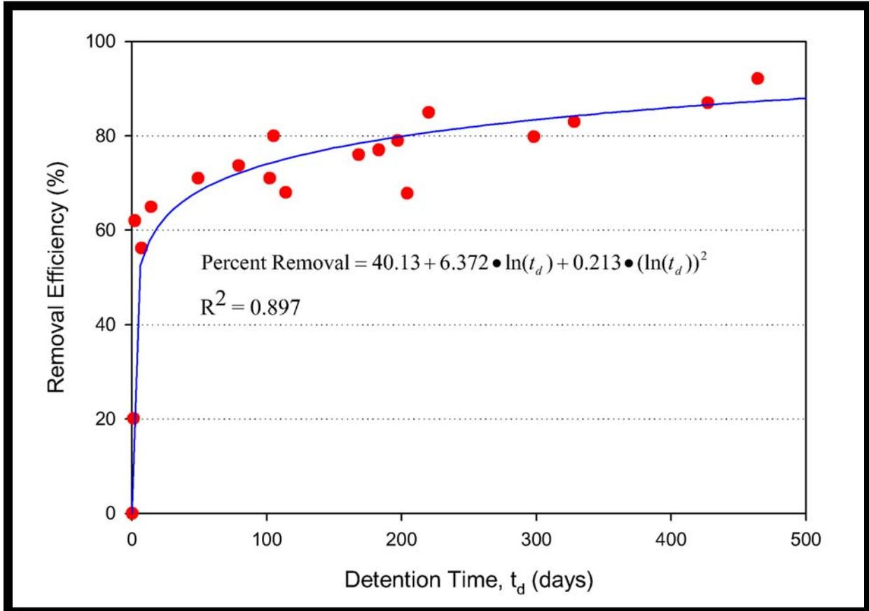
Exhibit 3. Phosphorous removal efficiency over time for a wet pond
