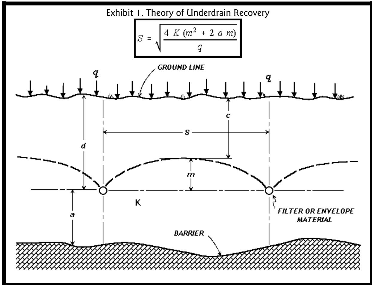
In the PONDS Underdrain module the input parameters, based on the formula in Exhibit 1, are expressed as shown in Exhibit 2 below. Note that the parameter  $d$  in Exhibit 1 is equivalent to  $H+t+D/2$  in Exhibit 2, and that this quantity represents the distance from ground surface (pond bottom) to the discharge control elevation (centerline of the drain pipe for free discharge conditions).
