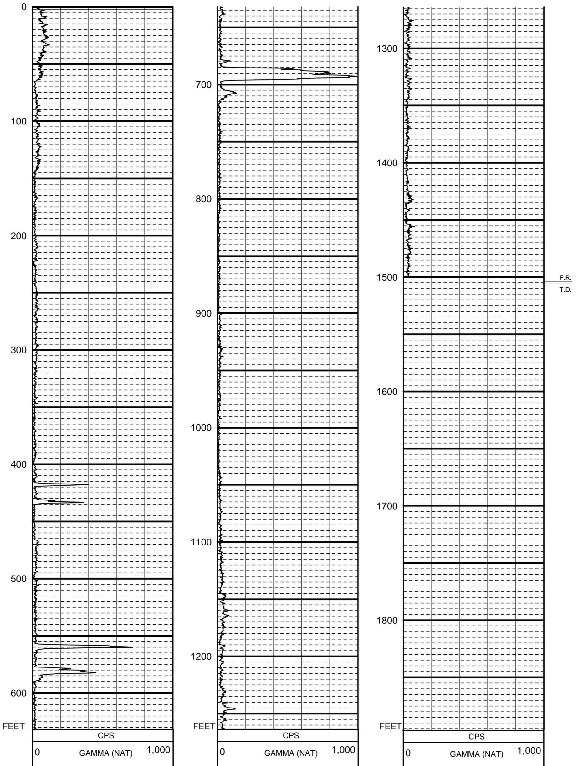
**Figure B-4.** Geophysical log collected in the exploratory core hole, between land surface and 1,505 feet below land surface, during exploratory coring at the ROMP 132 well site in Marion County, Florida. The logs were collected on 1/21/2009 using tool 9165C (caliper/gamma). The casing depth at the time of logging was 1,500 feet below land surface (see figure B-1). The vertical log scale is 2 inches per 100 feet.
