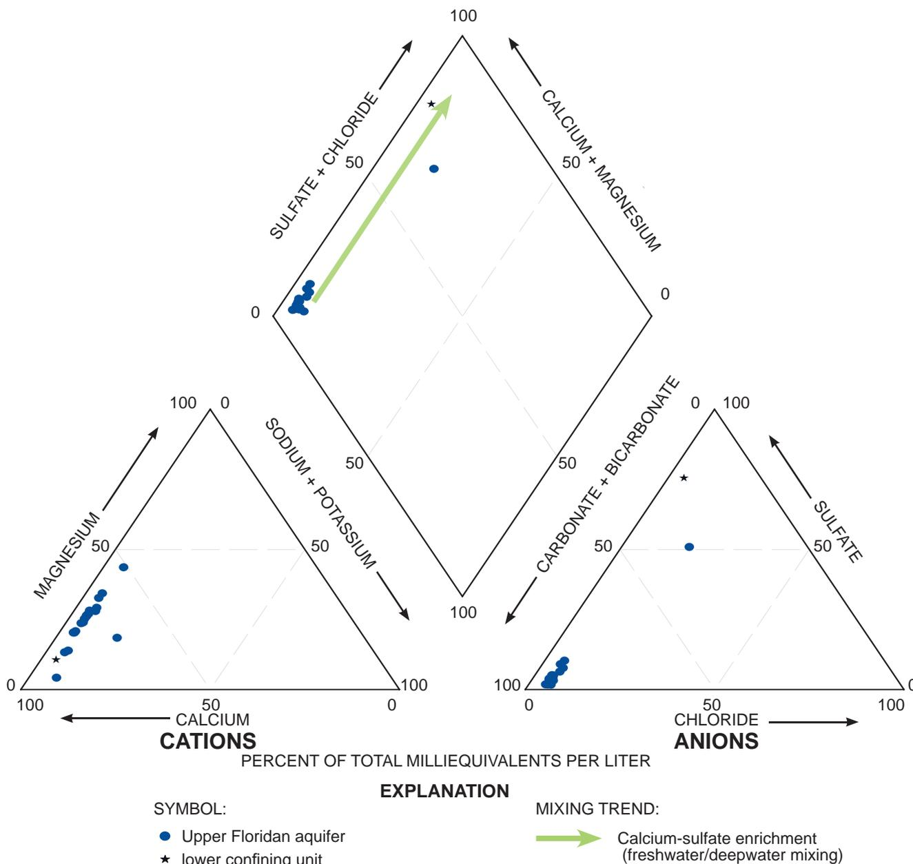
**Figure 9.** Piper diagram of groundwater quality samples collected at the ROMP 132 well site in Marion County, Florida.
