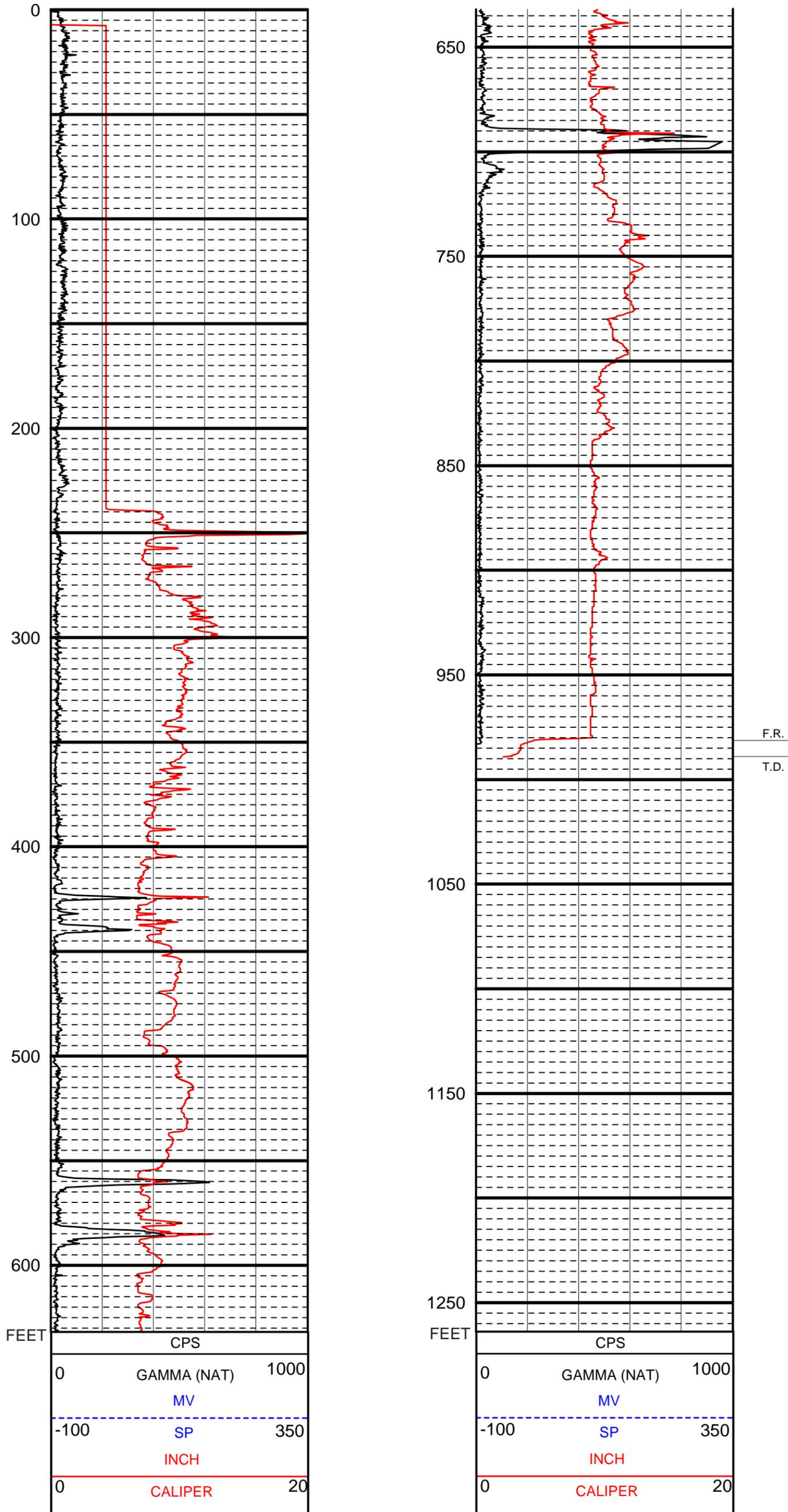
**Figure B-8.** Geophysical log suite collected in the permanent Upper Floridan aquifer monitor well, between land surface and 989 feet below land surface, after well construction at the ROMP 132 well site in Marion County, Florida. The logs were collected on 1/29/2010 using tool 9165C (caliper/gamma). The casing depth at the time of logging was 239 feet below land surface (see figure B-1). The vertical log scale is 2 inches per 100 feet.
