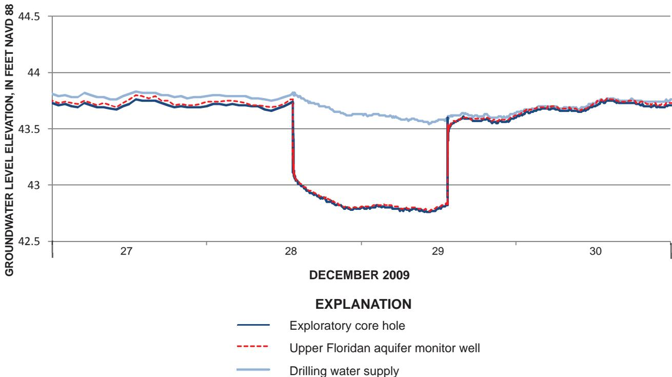
Figure 7. Hydrograph of groundwater levels in three wells before, during, and after the Upper Floridan aquifer performance test at the ROMP 132 well site in Marion County, Florida.
