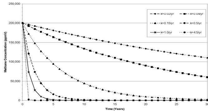
*Figure 1. Methane Concentrations versus time for variable degradation rates.*
